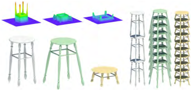
Figure 6: The original shape (in grey) has two deformed solutions which have almost the same compactness of stacking. The solution produced by our method (in green) keeps the original functionality and aesthetic appearance, while the solution generated by gap-function based method (in orange) loses most of the original functionality. Top left shows the gap functions of these three shapes.
