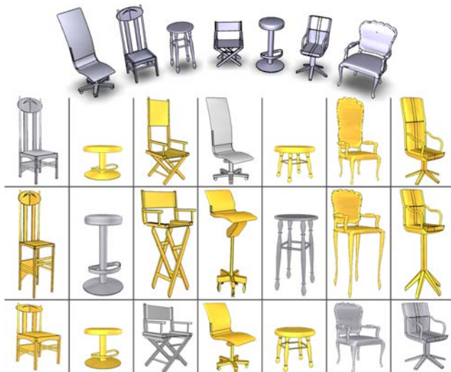
Figure 1: Style-content separation by anisotropic part scales facilitates part correspondence among a diverse set of chairs (top). The separation is shown by the table with rows representing identified styles. The correspondences allow automatic synthesis of novel shapes (shaded in gold) from the example set via style transfer.
