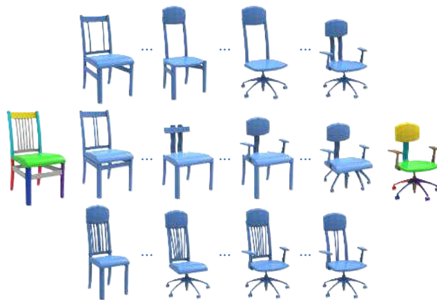
Figure 1: 3D shapes generated by topology-varying blending between a source (left) and a target (right), along three different blending paths. Part correspondence is shown by matching colors; some parts (neutral colors) are unmatched.
