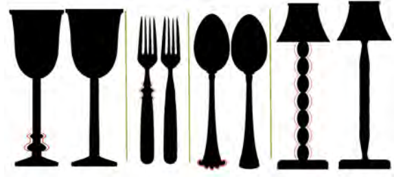
Figure 11: Style removal: the identified style-curves (red) are replaced by a smoothed style-less segment.
