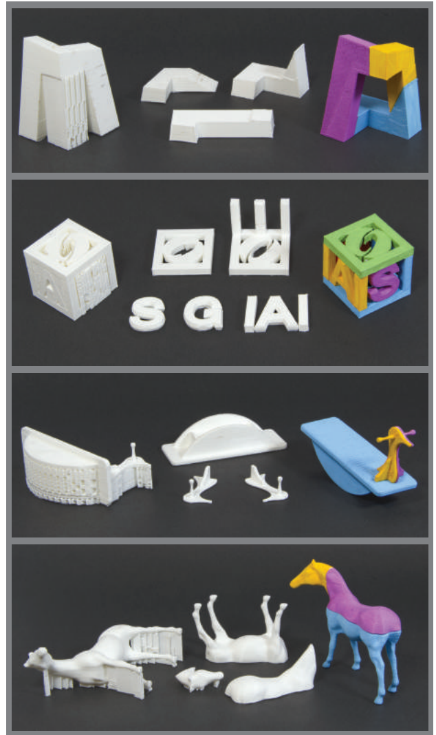
Figure 19: Photographs of some physically printed and fabricated 3D models. In each photo, from left to right, we show printed whole model, printed parts with bases lay on the ground, and the 3D model produced by gluing the parts which have been hand-painted in color. Note the printer’s ability to print slightly sloped geometry, e.g., on the CCTV model, so as to avoid some support material estimated in (5). Support material is noticeable as it is printed at a lower density. Also note support material interior to some shapes, e.g., the SIGA model, which would be hard to remove.
